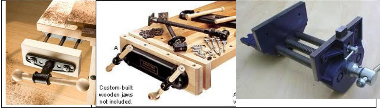
The shoulder vise (apparently more popular in Europe) is integrated into the bench top itself in an “L” shaped configuration while also requiring a fifth leg to support it. The shoulder vise excels in dovetailing because there’s no hardware in the way if you want to let a long work piece extend toward the floor. Shoulder vise kits are available from several woodworking suppliers.
