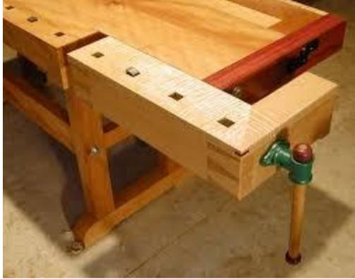
The tail vise nests into the front of the bench top, so it's designed in, not typically added-on. The tail vise is a surface-clamping design that holds stock between bench dogs. The moving jaw is surrounded by the bench top, providing excellent workpiece support. It resists sagging, unlike a cantilevered (shoulder) vise. Capacity is limited only by the length of the work surface, and since clamping force is closely aligned with the screw axis, the vise cannot rack.
