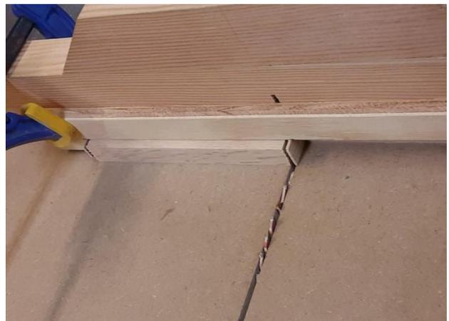
Last step for the tenons was cutting the cheeks, again accuracy and repeatability were important. Time to breakdown and purchase that tenon jig I've always wanted.
