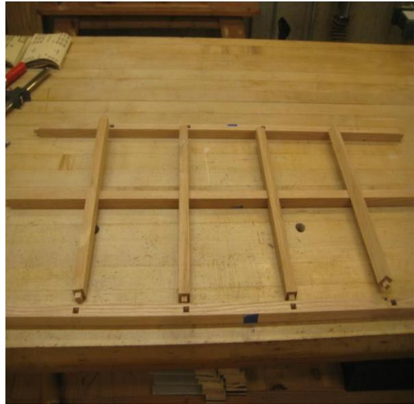
The next part was to set up and cut half laps and mortises for the long end rails. With 5 sections there were 2 set ups required, the 2 ends, and the 2 inside. Again this was done the same as the 2 end assemblies, but now there were 4 stiles to cut. Like the end assemblies it was all lay out, check and recheck dimensions, and patience!
