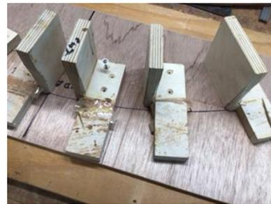
I ripped thin strips of cherry, longer than needed, keeping them in the correct orientation and placed 5 strips on the bending jig, added glue, tighten the clamps, and left overnight. I made two extra legs to be used between the lower and upper top.
