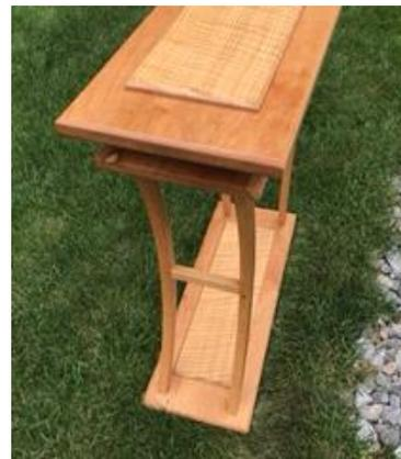
I finished using two applications of watered down Hide glue on the oak due to its porous nature, an application of Seal Coat and several coats of satin General Finish Arm-R-Seal.
