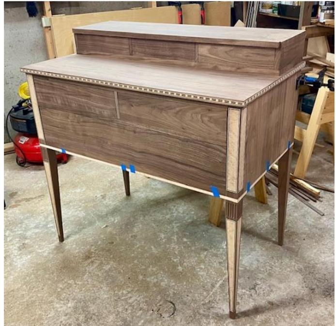
I applied the Birdseye maple veneer to the drawer faces with a hammered hot hide glue technique. The perimeter of each drawer has cross grain walnut with holly and ebony banding. Cutting and fitting the 45° corners was challenging.
