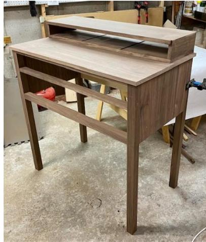
The sides are mortised and tenoned into the rough legs. The front 2" wide rails are twin tenoned to the legs. The small cabinet at the top will hold three small drawers. I made a practice leg to work out how to build the Birdseye Maple veneer and the ebony and holly stringing. I made the veneer slightly wider than the finished width, then cut a 1/8" wide slot for the stringing with a micro fence system on my small router.
