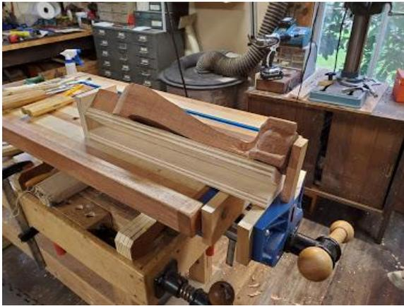
*A cradle to hold the leg for excavating the webbing.*
