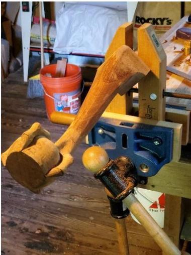
*A modified hand screw helps when rounding the leg with rasp, spokeshave, and files.*
