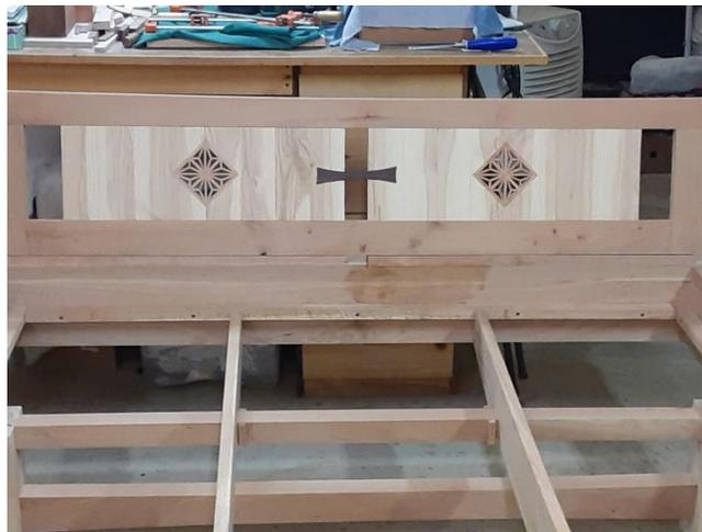
With the headboard assembled and attached, all that was needed was a finish sand, note messy glue spill on bed side and riser board. Final finish is first coat of boiled linseed oil to bring out wood and grain pattern; 3 coats of clear shellac (why just do one when 3 is just a little more time); and finally several coats of furniture wax, rubbed out with white non-woven abrasive pads.
