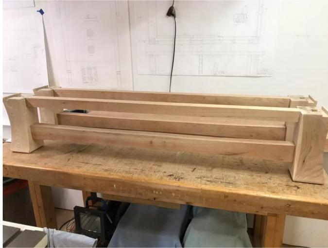
The stretchers are 2 by 2 cherry mortised into the legs. The bottom stretcher has top and bottom curves to match the top of the head board, hard to see with the frame all assembled, but I'll know. The outside dados on the leg tops match the width of the bed frame rails to position it in place.
