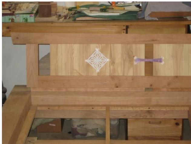
The head board is made with 1" thick cherry. Assembly is all mortise and tenon with the ash panels set in dados in the top and bottom rail. An 11° angle was set on the headboard from the riser board between the bed rail and headboard. The riser board is set in place with glue and screws; mortises on the riser board were used to locate the tenon's on the bottom of the headboard.
