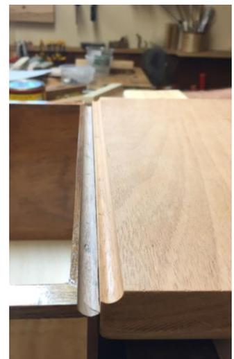
Grooves of box (L) and lid (R) made at the router table to hold the wood hinge
