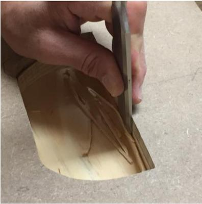
Using a form for cleaning the recessed area on prototype stock
