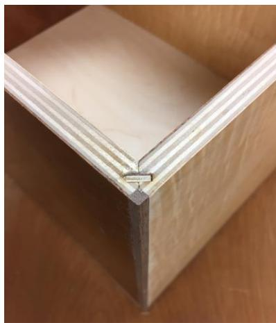
Mitered cuts and vertical spline join the sides. Walnut corners protect the veneer edges.
