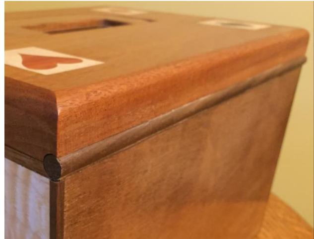
The wood hinge composed of five dowels glued in routed grooves (see picture above this one). The short metal rod segments joining the dowels cannot be seen.
