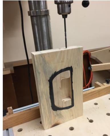
Drill hole through the side of the prototype lid for handle
