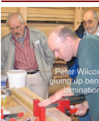
Peter Wilcox demonstrating bent lamination.
