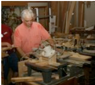
Joe Aeillo and one of his many ingenious devices; a coping machine for cope and stick doors
