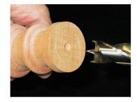
For the reeded section you will need a rough leg blank at least 4" longer than the expected reeded length. This is to allow for the dowel tenons after the reeded portion is finished. The blank's square should be at least 3/8" larger than the final maximum diameter to allow for roughing to the starting diameter. Rough turn the leg to a straight cylinder.
