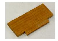
To set the guide rails, first mark the jig's top edges at the location of the top and bottom cylinders cut for the rough turning. Insert the gauge as shown at the right with the narrow edge resting on the top turned cylinder. Raise the guide rails to touch the notches in the gauge and tighten. Repeat the steps at the lower turned cylinder and set the rails. They are now parallel to the desired taper of the leg. Double check these adjustments.
