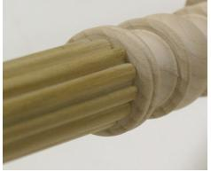
The three parts of the leg are shown above. The top (pilaster end) and foot are conventional turnings with a bored mortise on the mating end of each. The centered tapered section has turned tenons to mate with the top and foot. Note how cleanly the tapered reeds dive into the surface of the bead. This is a major time saver over hand scraping the reeds and carving the interface.
