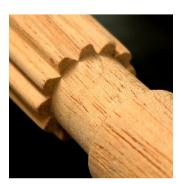
You will now need to scrape and sand the reeds to obtain a pleasing shape. An old fashioned "church key" with a small circular shapes filed on either side of the point works very well. It is easy to hold to remove and round the flats. Finish with sandpaper folded sharply to insert into the grooves.
