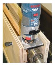
If all went well, you should have reeds ending at the top and bottom as shown below. These are straight off the router. After you rout the remaining legs, you can then remove the jig from the lathe.
