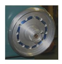
Unplug your lathe for safety and set the index wheel for the first reed. With the router placed over the bit relief section at the foot, rout the first reed with a slow, firm motion of the router. Do not stop moving the router, or you will end up with burn marks on the reed. Reset the index and repeat until twelve reeds have been cut.
